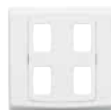
S8824 WHI 4 gang including earth terminal (For 20AX, use switch module SX8423X, with max. 2 nos only)
