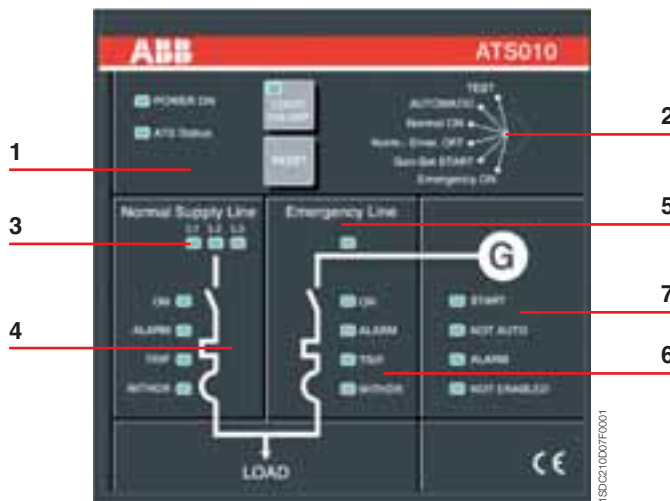
Caption 1 Status of the ATS010 unit and logic 2 Operating mode selector 3 Normal line check 4 Normal line circuit breaker status 5 Voltage on the emergency line 6 Emergency line circuit breaker status 7 Generator status
