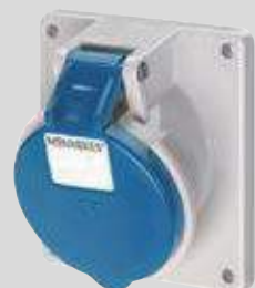
Panel mounted receptacle screwless, with TwinCONTACT, flange 16 A, 3 p: 73.5 x 64 mm, 16 A, 4 + 5 p, 32 A: 100 x 92 mm, inclination 20°, 32 A: optional fitted with auxiliary contact
