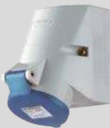
Wall mounted receptacle screwless, with TwinCONTACT, suitable for through wiring, internal fixing, 4 p and 5 p receptacles the enclosure can be turned 180°
