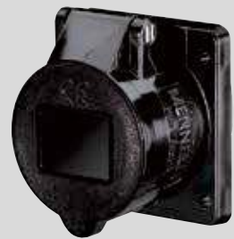
Panel mounted receptacle straight, flange: 72 x 65 mm, fixing hole spacing: 52 x 52 mm
