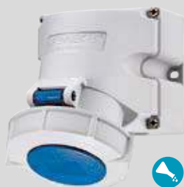
Wall mounted receptacle screwless, with TwinCONTACT, highly resistant to chemicals, suitable for through wiring, with 2 external fixing points, receptacles are designed for adding an auxiliary contact switch, enclosure base can be turned 180°
