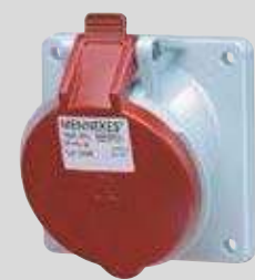
Panel mounted receptacle screwless, with TwinCONTACT, standard flange dimensions 85 x 85 mm, 20° inclination, optional fitted with auxiliary contact
