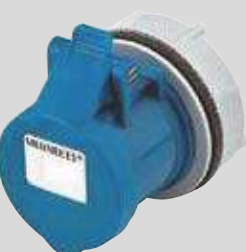
Panel mounted receptacle RAPIDO screwless, with TwinCONTACT, with central locking system, round flange for central fixing, diam. 61 mm
