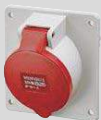
Panel mounted receptacle standard flange dimensions, uniform fixing hole spacing, 15° inclination for 16 A and 32 A, 20° inclination for 63 A
