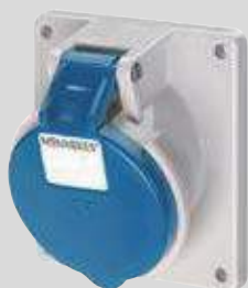
Panel mounted receptacle flange 16 A, 3 p : 73.5 x 64 mm, 16 A, 4 + 5 p, 32 A: 100 x 92 mm, inclination 20°, 32 A: receptacles optional fitted with auxiliary contact
