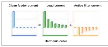
An ABB active filter is a power electronics based electrical equipment that is installed parallel to the polluting loads. It monitors the line current harmonics, as well as the customer requirements programmed by the user. It can then generate for each harmonic frequency a compensation current in perfect phase opposition to the polluting current.
